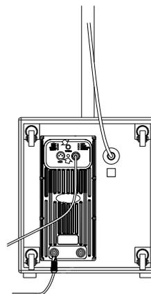
Making sure that the volume is turned down, switch on the system using the switch on the back panel. Select the preset you need and adjust the volume to the desired level\*.
