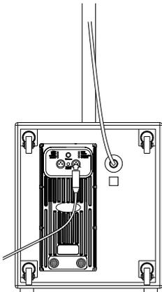
Connect the subwoofer to your sound source via the line input socket on the panel.
