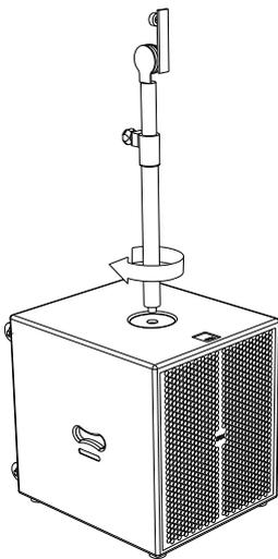
Take the connection stand and screw it into the hole on the uppermost part of the subwoofer.
