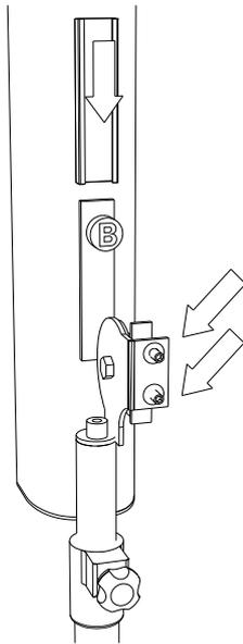
Take the K4m TOP and insert it into the connection stand, by inserting the speaker fixing plate into the coupling plate. Tighten knob B on the coupling plate. If necessary, adjust the angle of the K4m TOP by holding it with one hand and loosening knob C with the other. Do not tilt the loudspeaker more than 10°.
